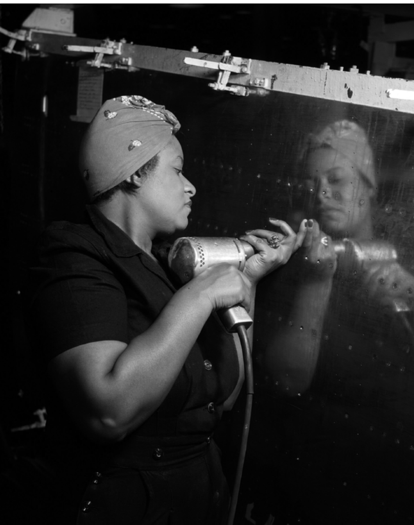
A REAL-LIFE "ROSIE THE RIVETER" OPERATING A HAND DRILL AT VULTEE-NASHVILLE, TENNESSEE, WORKING ON AN A-31 VENGEANCE DIVE BOMBER IN 1943. PHOTO BY ALFRED T. PALMER, PUBLIC DOMAIN.
